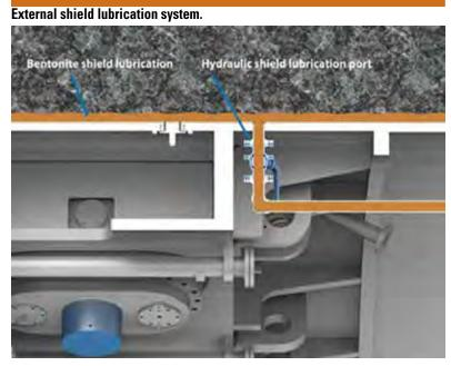
Field results have shown, time and again, that a TBM built with risk insurance-type features (such as probe drills, shield lubrication, etc.) can have a huge impact on a project's success in terms of schedule, cost and safety. It is better to build features into the machine from the start as part of a comprehensive risk management strategy, than to add them in the tunnel after an unforeseen event has occurred or the machine has become stuck.
