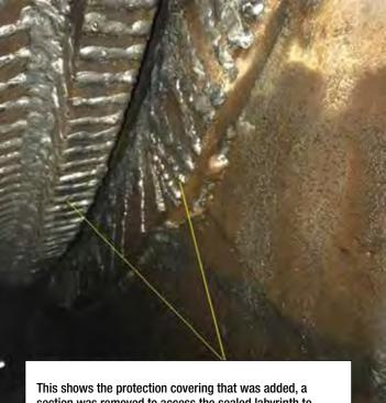
section was removed to access the sealed labyrinth to assess the extent of the damage.
